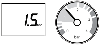
Fig.52 Restore water pressure
